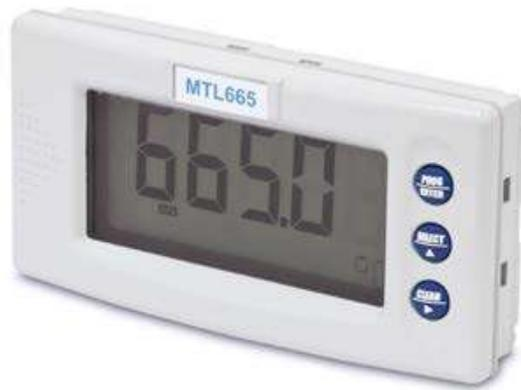
The MTL665 is a DIN-standard, panel mounting, IS indicator to display the current flowing in a 4–20mA loop. The small voltage drop of <math><1V</math> allows the loop powered display to be installed in almost any 4–20mA loop.
