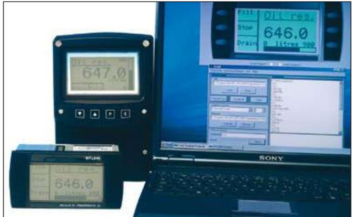
**The MTL646/647 serial text displays** are intrinsically safe instruments that can display text and simple graphics in a hazardous area. Having a number of push-buttons and two solid-state switched outputs, they provide a low cost operator interface ideal for simple machine and process control applications. In addition to new installations, the legacy protocol enables existing MTL643/644 display systems to be easily upgraded.
