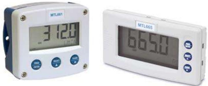
The **MTL661, MTL662, MTL663 and MTL665 digital indicators** enable process variables to be displayed locally in hazardous and general purpose plant areas. A typical example would be the re-transmission of mass/flow computations from the safe area, through a suitable MTL IS interface to the indicator in the hazardous area.
