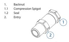
421/2K size only. View for clarity only, do not disassemble ① & ②.
