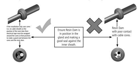
Do not disassemble the gland to inspect the Resin Dam, diagrams are for representation.
